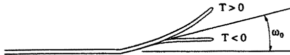
Fig. 16. Crack growth behaviour influenced by non-singular T stress at the crack tip.
